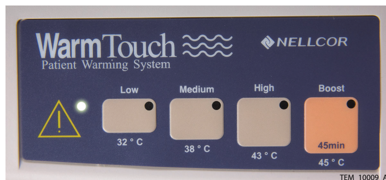
Figure 3. Control Panel Warning Indicator and Temperature Selection Keys
